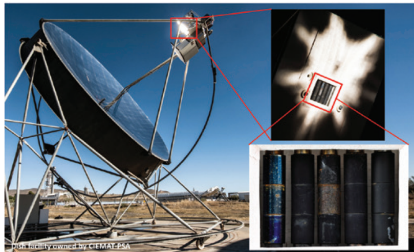
Fig. 2: Accelerated aging testing of different absorber coatings in the dish concentrator test bench at Plataforma Solar de Almería.
