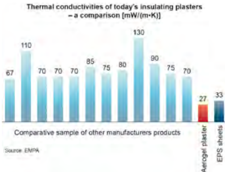
Figure 2: Comparison of the thermal conductivity of conventional insulating renders with the Empa/Fixit Aerogel render
