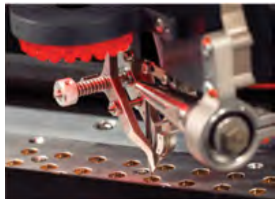
Fig. 3: Automatic packaging of laser power converters on transistor outlines at Fraunhofer ISE: thin wire bonding for electrical contacts.
