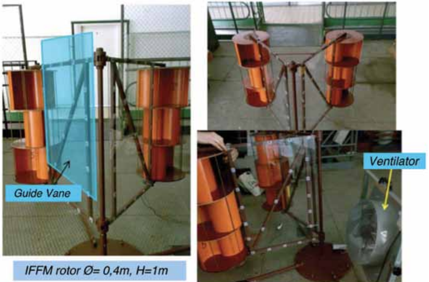
Fig. 4. Small wind turbine (P= 2 KW) elaborated in IFFM Laboratory. IFFM patent pending design.
