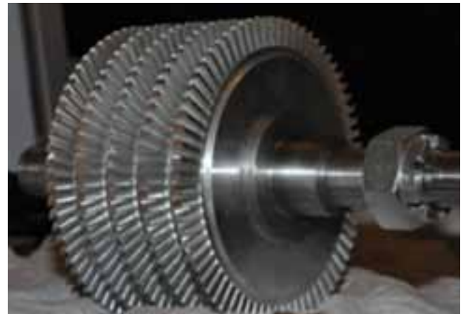
Fig3. The rotor of the micro-turbines (P=3 KW, N=8000 rpm) and new generation of biomass boiler (20 KW) tested in IFFM laboratory of the Polish Academy of Sciences.
