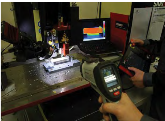
Thermal measurement of the THERMACO demonstrator
