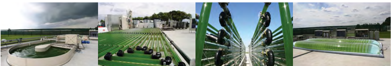
Figure 2: The four types of reactor systems at AlgaePARC (left to right): open raceway pond, horizontal tubular reactor, vertically stacked tubular reactor and flat panel reactor
