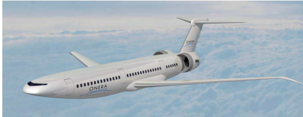
NOVA configuration with semi-buried engines for boundary layer ingestion
