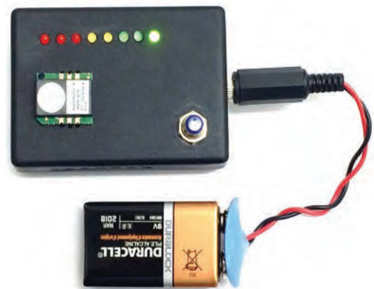
The demo device features AppliedSensors' iAQ-engine as gas sensor module which can be operated with an external power supply or 9V battery. Changes of VOC and hydrogen concentrations are indicated by LEDs and can be logged via USB or memory card. A BMS can be interfaced via I/O pins and I2C bus.
